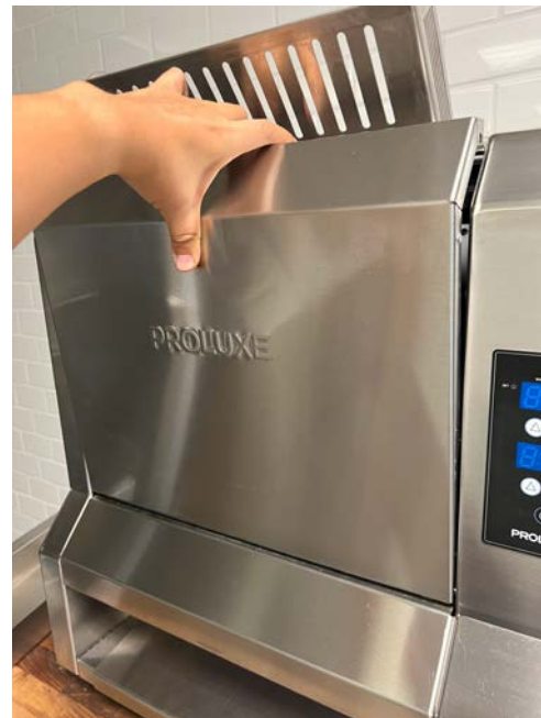
IMAGE 4: LIFT FRONT COVER TO INSTALL FEEDER
