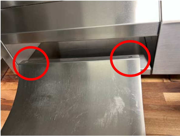
IMAGE 1: RAMP SIDE WITH HOLES GOING INTO THE TOASTER
